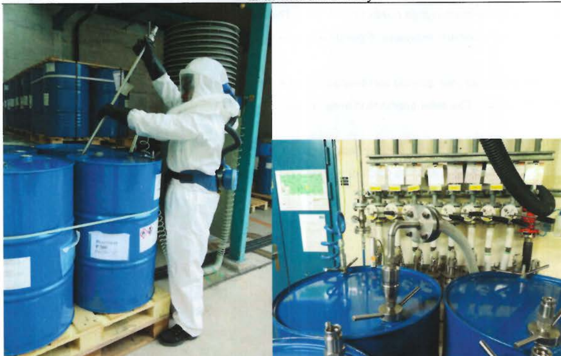
Figure 1: Use of suction lance at the production facility, with connected piping and storage drum
