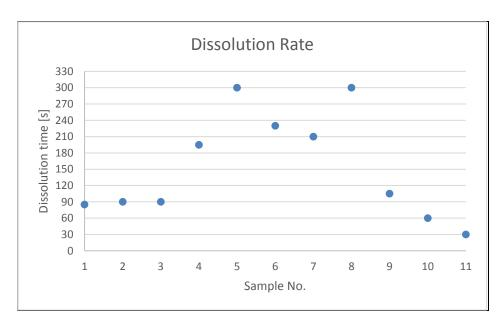
The time for the capsules to dissolve in water at 20 °C differs from product to product. EC Regulation no. 1297/2014 stipulates that this must be at least 30 seconds.
