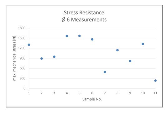
The maximum mechanical stress that the capsules withstand under standard conditions differs greatly from product to product. EC Regulation no. 1297/2014 stipulates that this must be at least 300 N. Unfortunately, neither the test protocol nor the evaluation is specified in the text. For example, it is not clear whether the maximum mechanical stress for ALL capsules of a product, or the mean of a measurement series should be greater than 300 N.
